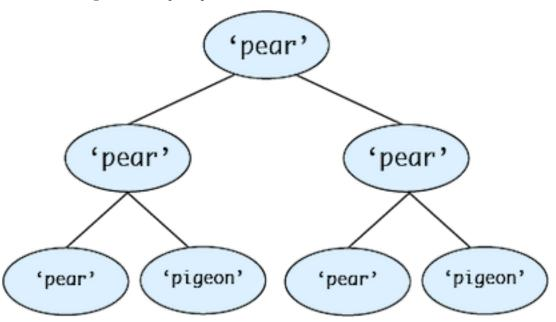
The function returns a list of locations of pigeons in t, where each location is a two-element list with the "depth" as the first element and the "left" as the second element.
